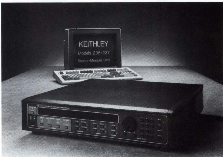
Combining a 4-quadrant V/I source with an electrometer and a DMM in a 3½-in.-high single-channel package, Keithley's Model 236 and Model 237 source/measurement units are fully programmable via IEEE-488. They provide an economical solution to many test problems.
