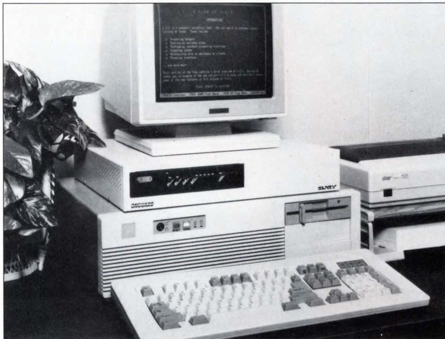
Fitting between a PC's monitor and base unit, the SL-400 uninterruptible power supply from Clary Corp provides 30 minutes of backup power for two IBM PCs or compatibles.
