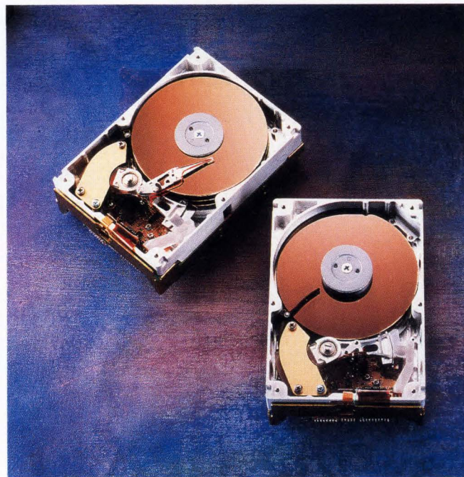
A multisegment caching capability effectively reduces the average seek time by as much as 50% in Quantum's ProDrive series of 3½-in. drives, which range in capacity from 40M to 170M bytes.
